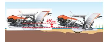
The auto sensor detects undulations to adjust the machine height up to 450mm contributing to efficient operation even in deep paddy fields.
