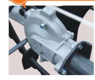
The axle case has been changed from a grease method to an oil bath method to improve maintainability and durability.
